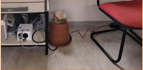
Indicative images from the installed seismographs of the temporary network for monitoring the postearthquake sequence of the Tyrnavos – Elassona earthquake.
