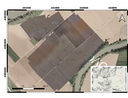
▲ Orthorectified image of the liquefied areas (gray spots). Images from a series of high flying UAV campaigns have been combined with orthophotos from the Cadastral project of Greece.
