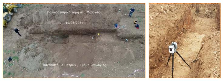
Palaeoseismological trench from above. Drone footage of the California style trench at Meschori area and LiDAR mapping of the excavated trench
