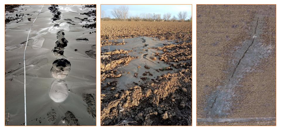
Liquefaction phenomena were also generated in the southwestern part of the affected area. More specifically, in the Pineios River bed from Pineiada to Farkadona. They comprise sand boils along ground cracks with length up to 60 meters. They are attributed to the lithology of the river deposits, the shallow water level in the river bed and to the intense earthquake ground motion.
