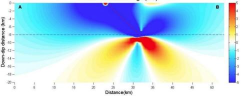
The seismic fault model (seismic source) of the mainshock is based on the GFZ's moment tensor solution (strike, dip and rake), the scalar relationships of Wells & Coppersmith (1994; length and width), and the interferograms along with the site observations (position).
