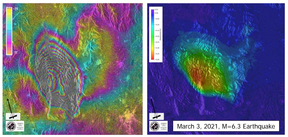
A co-seismic interferogram and displacement map was generated using the Ascending geometry (Orbit: 102, Master: 25/02 16:24:15 GMT, Slave: 03/03 16:23:34 GMT) in the GAMMA software. The displacement map shows subsidence up to 40 cm and uplift up to 3 cm, after the Mw=6.3 earthquake including all the seismic events between 25/02 and 03/03.
