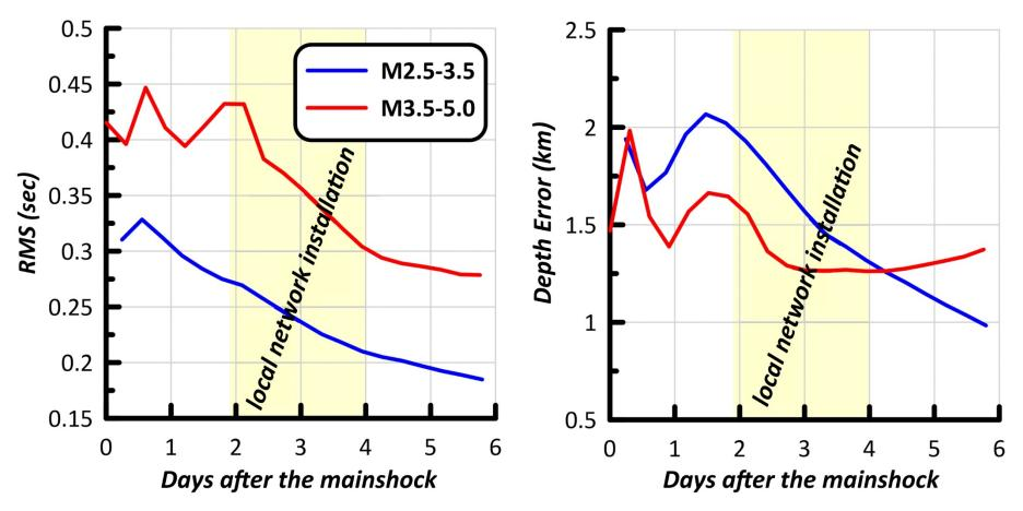
Smoothing variation of the mean square error of travel times (RMS) and the standard depth error of the postearthquake sequence of the March 3, 2021 earthquake. The  $\sim$  450 epicenters of earthquakes with M> 2.0 are also presented.
