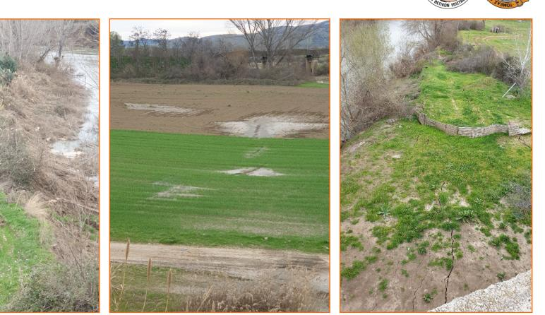
(Left) Lateral spreading along the Pineios River banks, (middle) liquefaction phenomena in the fields close to Pineios River and (right) ground cracks arranged parallel to the Pineios River. It is significant to note that these secondary earthquake environmental effects were observed close to the bridge of Pineios River located close to the Koutsochero village. The bridge suffered cracks and damage due to seismic pounding between bridge segments.
