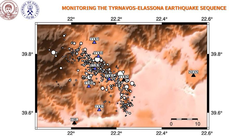
Spatial distribution of the permanent (black triangles) and temporary (blue triangles) seismic monitoring network of the post-seismic sequence of the Tyrnavos-Elassona earthquake. The ~450 epicenters of earthquakes with M>2.0 are also presented, for which there are solutions by the analysts of the Seismological Network of the Aristotle University of Thessaloniki.
