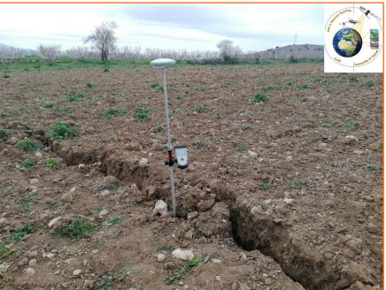
The fault trace was mapped by RTK GNSS receiver
