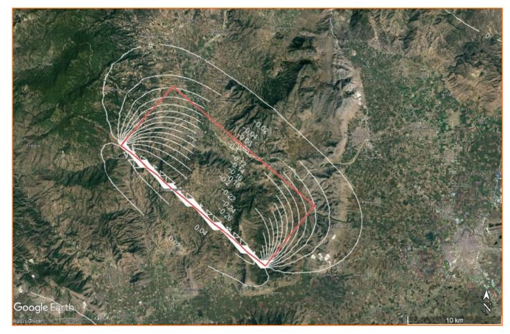
A preliminary model of the seismic source is showing vertical displacement on the ground
