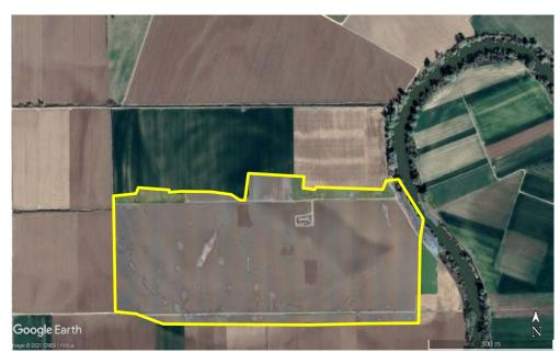
▲ Comparison with current and historical satellite images, show that in the area of Pineios river the liquefaction is clearly associated with older abandoned meanders of the river, indicating a differentiated composition, more susceptible to liquefaction
