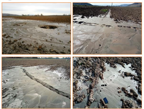
More typical examples of the generated liquefaction phenomena in the southwestern part of the affected area. Large craters were formed, from which the liquefied material has been ejected and partially covered the adjacent field. The extend of the liquefied material indicate the intensity of the earthquake ground motion.
