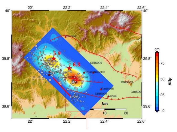
Estimated fault length associated with the March 3, 2021, M=6.3 earthquake of the order of 15 to 17 km.
