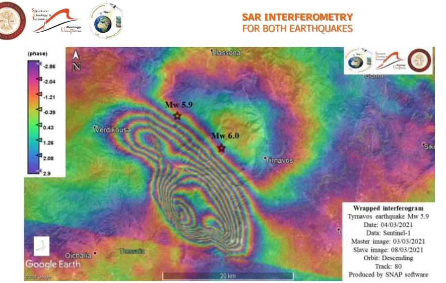
Wrapped interferogram of the two earthquakes produced by SNAP software
