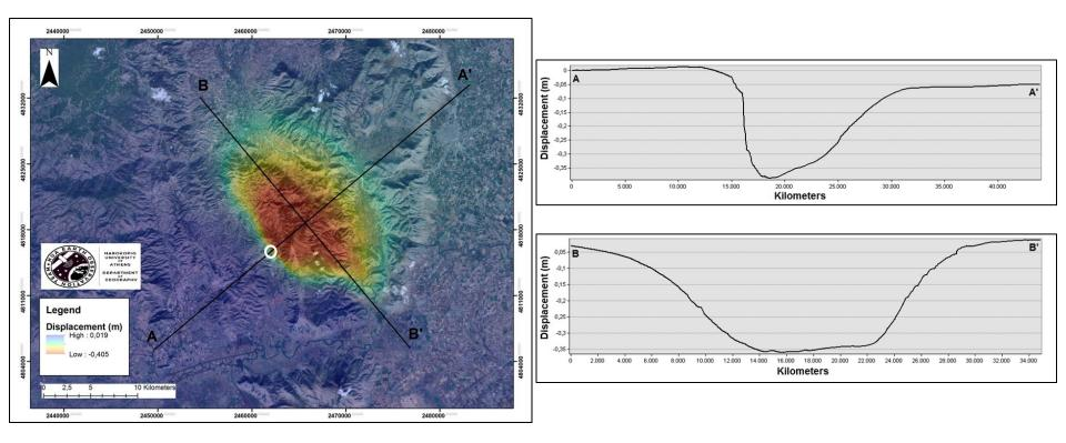
Two sections were generated in order to visualize the ground deformation due to the Mw=6.3 earthquake. It is notable that in the 15 km of the AA' section, the subsidence is very abrupt.
