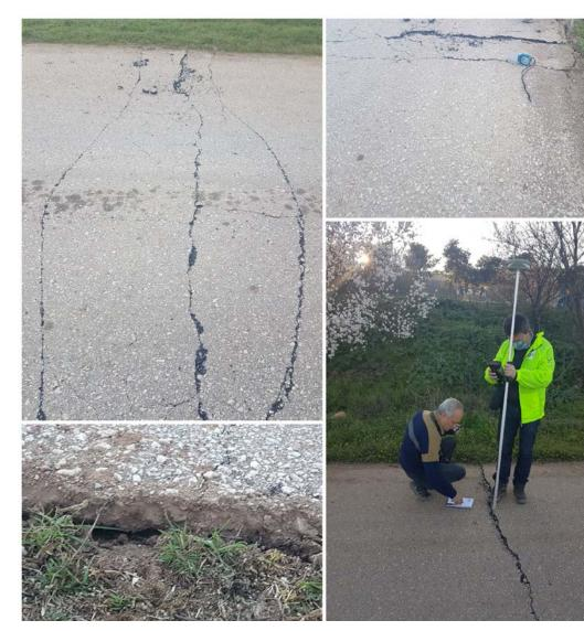
Mapping extensive ground cracks generated by the March 3, 2021, Mw=6.3 earthquake near Damasi village
