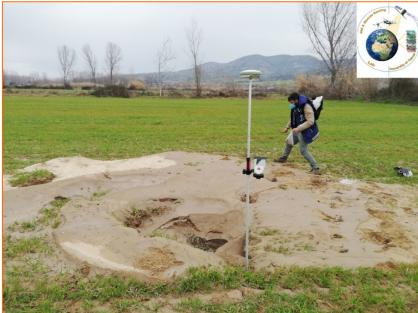
The scientific team of the University of Patras (Koukouvelas, Nikolakopoulos, Kyriou, Apostolopoulos, Zygouri, Verroios, Belesis, Tsentzos) mapped with UAVs and RTK GNSS receivers several ground cracks and liquefaction phenomena in the broader area of Damasi, Mesochori and Vlachogianni.
