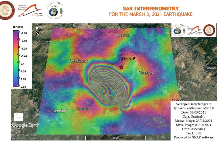
The scientific team of the University of Patras combined laboratory work and field mapping. Sentinel-1 data was processed and interferograms were produced by SNAP software.
