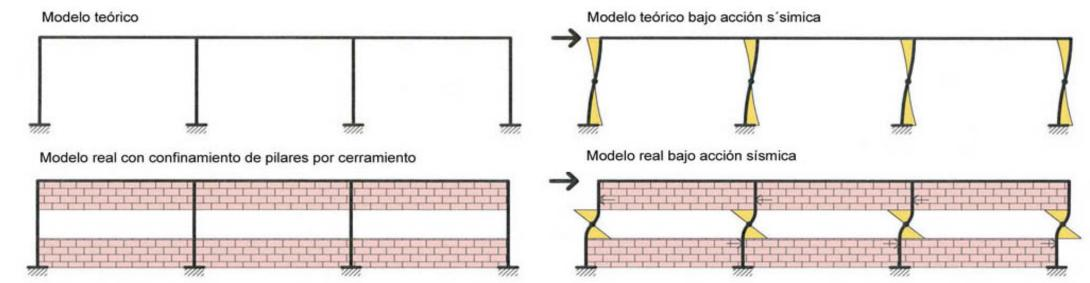
Captured column; the expected performance of a column as foreseen on top is compromised by the restraining action of the partitioning brickwork, resulting in a 5.1.3 'shorter' column taking on all the shear force.
