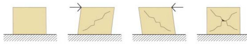
Model of shear damage formation. 3.4.4
