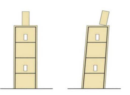
Scores of mosque minarettes were subject to strong shaking 9.1.1 in the epicentral area which justifies their inclusion in this report; A simple model for non-structural damage to the mosque lantern is shown above. All mosque minarettes are built to similar geometric specifications; a RC frame with no diaphragm action save for the spiral stairs. Lantern is a non-structural element on the roof.
