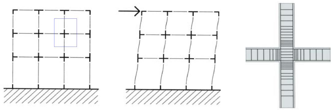
4.1.2 This is good practice; In a moment resisting frame, column to slab and beam connections are carefully detailed for rigidity, stiffness and full coupling action between members. A more equal size distribution between vertical and horizontal elements is designed to invoke deflection away from connections. There is no evidence that these conceptual principles were applied in recent RC frames in Al-Hoceima.
