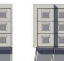
**4.9.5** Failure model; Very stiff upper floors drift over an open plan ground floor with insufficient resistance to
