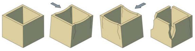
The cyclic reversal of strain in two perpendicular walls meeting at a corner causes brittle 3.5.4 failure in unreinforced masonry construction resulting in this widespread earthquake damage.
