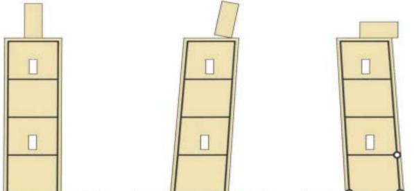
Failure model; In this example incipient plastic hinging is observed in base of tower. 9.6.1
