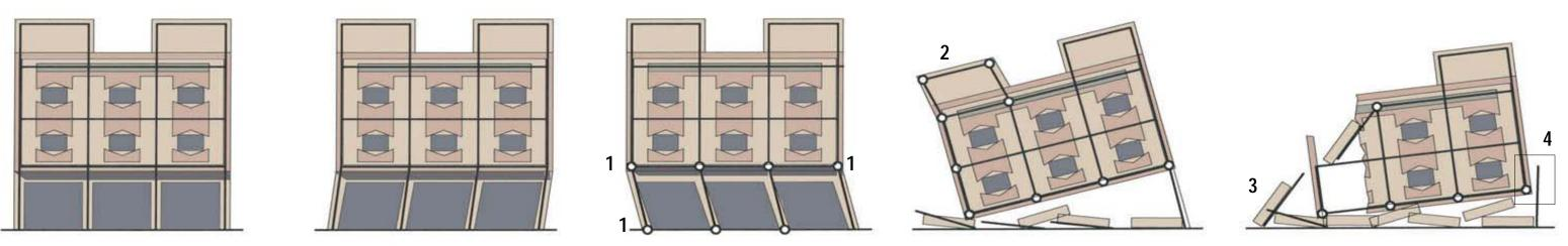
7.2.4 Failure model, Open plan shops and densly compartmented flats above result in a soft storey situation. Beyond the lilmited elastic range of the column to slab connections, plastic hinges are fomed. (1) With reduced stiffness, plastified connections fail, throwing the building to the ground left side first. (2) Impact with the ground probably causes the failure of the left tower and its roof falls to the road.(3) The last column to detach is n°4 (4) settling the building on its own scree.
