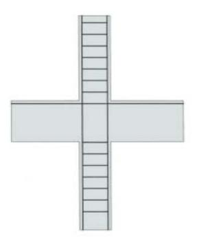
4.1.1 Ths is poor practice; Vintage concrete structures and those which do not incorporate seismic resistant design criteria have poor column to beam and column to slab connections. With emphasis on design for static loads, slabs tend to be very stiff and much more stronger than columns. Columns deform and plastify long before beams or slabs. The majority of buildings analysed in Imzuren were of this kind.
